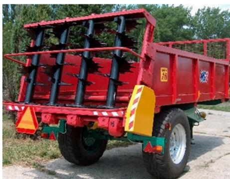
Fig. 1. Rear delivery vertical-axis beaters MG5
